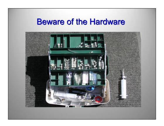
The tackle box on the left shows the required hardware to collect soil gas samples in Summas.
